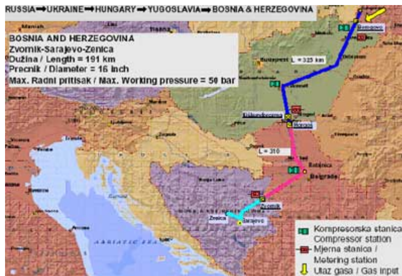
Figure 2 The gas supply system in B&H
